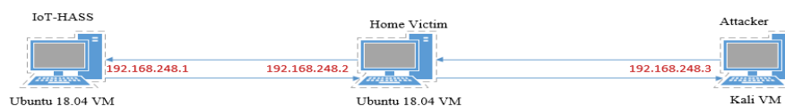
Figure 39. IoT-HASS Running in Passive Mode as an IDS Inside a VM Environment
